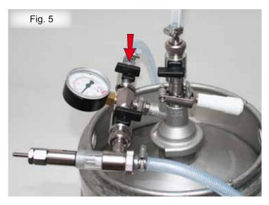
When the correct pressure (about 1 bar) shows on pressure gauge close ball valve I.
