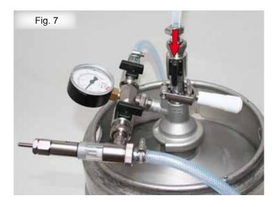
Open ball valve III (beer supply). Pump pressure in the beer line must be approx. 2.5 bar.
