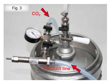
Connect filling head to keg and pull/press the handle down to activate.
