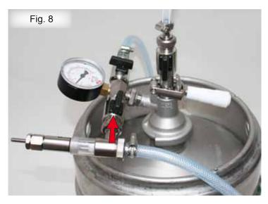
Open ball valve II (CO<sub>2</sub> line). CO<sub>2</sub> vents until non-return valve closes. Keg is now full.
